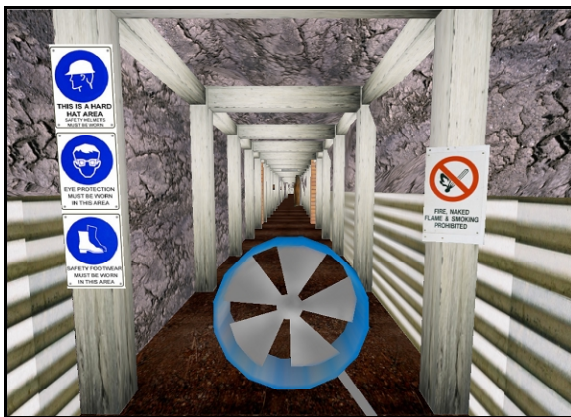
Figure 5. Navigating around UQEM with a vane anemometer for conducting a quantity survey
