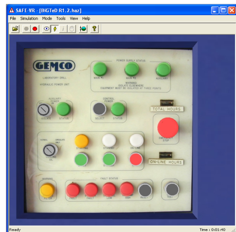
Figure 9. Control interface of power pack
