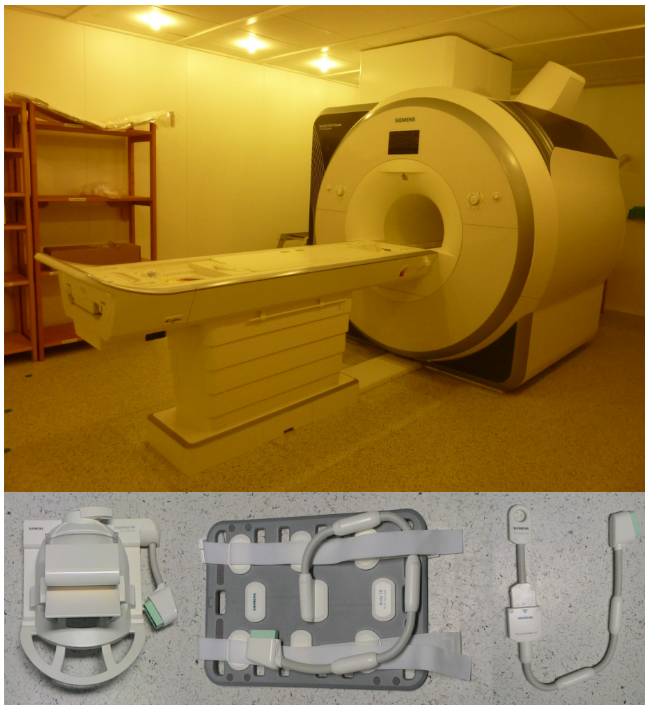
Figure 5.1: (Top) MRI system and (Bottom) receiver coils. (Bottom left) 64-channel head coil, (bottom middle) 18-element thorax coil, (bottom right) single-channel loop coil.
