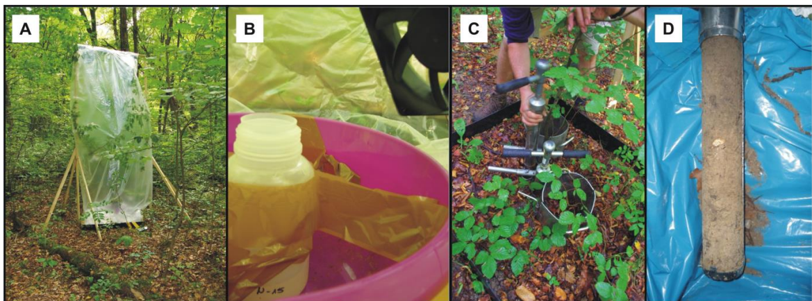
Figure 1.3-4: Chambers that were used for simultaneous in situ 13 CO 2 pulse labeling of 20 replicates per tree species (A). Ventilation system inside the chamber (B); split tube for soil sampling with three replicates per tree (C), 7 cm soil cores taken subsequently from the soil surface down to 30 cm depth (D).
