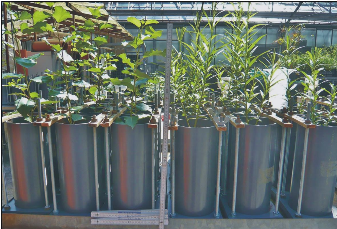
Figure 1.3-6: Setup that was used for ^{15}\text{N} labeling of willow and poplar cuttings with ^{15}\text{NH}_4\text{NO}_3 , \text{NH}_4^{15}\text{NO}_3 and reference treatment with \text{NH}_4\text{NO}_3
