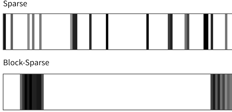
Figure 3.1. – Sparsity differs from block sparsity. A sparse vector contains only few entries different that zero distributed along the vector. Instead, a block sparse vector is composed by few blocks of non-zero entries.
