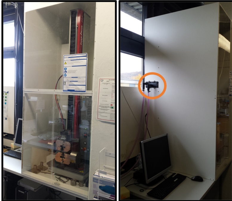
Figure 7-1 Photographs of the cooling casing that was constructed by the workshop. In the right photo, the position of the air conditioning is highlighted.
