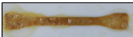
Figure 3-8 Photograph of an inhomogeneous dogbone specimen.
