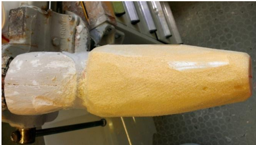
Figure 21 – Positive cast with a thermoplastic liner still attached and polished polyurethane extension pre-shaped to provide a solid base for casting the outer semi-permanent socket
