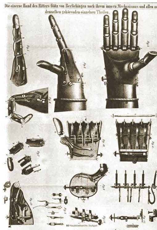
Figure 1 – Schematic representation of parts belonging to Götts von Berlichingen's hand (16th century), an early iron prosthetic substitution for a transradial amputee. Even though passive, its fingers can be prepositioned and latched in order to offer certain degree of functionality in combat. © |2006 |de.wikipedia-commons
