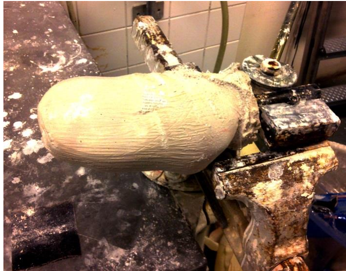
Figure 19 - Positive cast after molding ready for refinement and polishing. Strong anchoring line across the front of the elbow can be observed.
