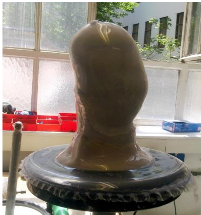
Figure 20 - Warmed up thermoplast has to be carefully applied on the positive in order to ensure tight and comfortable fit. This is being done using a vacuum pump during gentle and slow stretching of the material.
