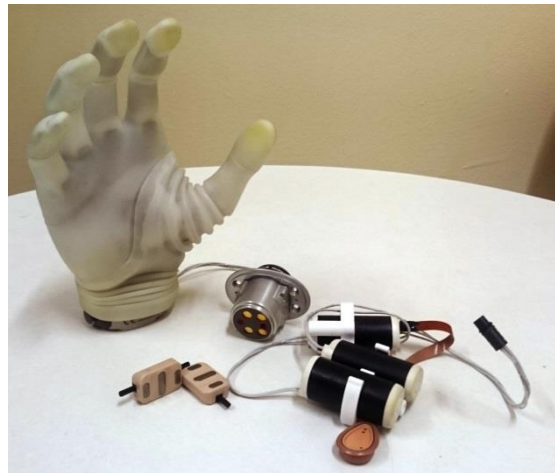
Figure 3 – Advanced prosthetic hand – Michelangelo, Ottobock Healthcare GmbH - with a rotation unit, extra battery pack and a pair of surface EMG electrodes. This particular prosthesis has an actuated thumb which allows it to close in two ways: pinch grip and key grip.
