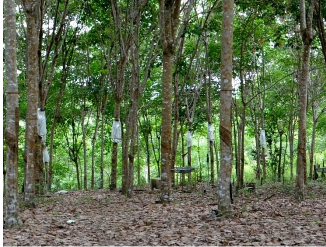
Figure 2.3 Field installations of TDP measurements on rubber trees in the long-term monitoring rubber plot.
