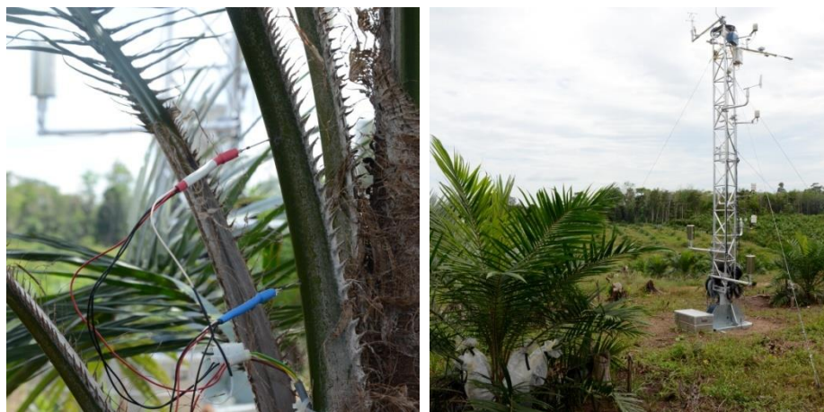
Figure 2.4 Parallel sap flux and eddy covariance measurements in a young oil palm plantation.
