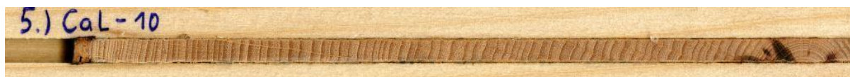
Figure 3.1 Example of an increment core, mounted on a wooden groove board (from the loamy field site in Calvörde).
