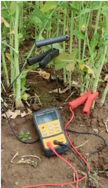
Fig. C 5: Measuring set-up for electrical capacitance
