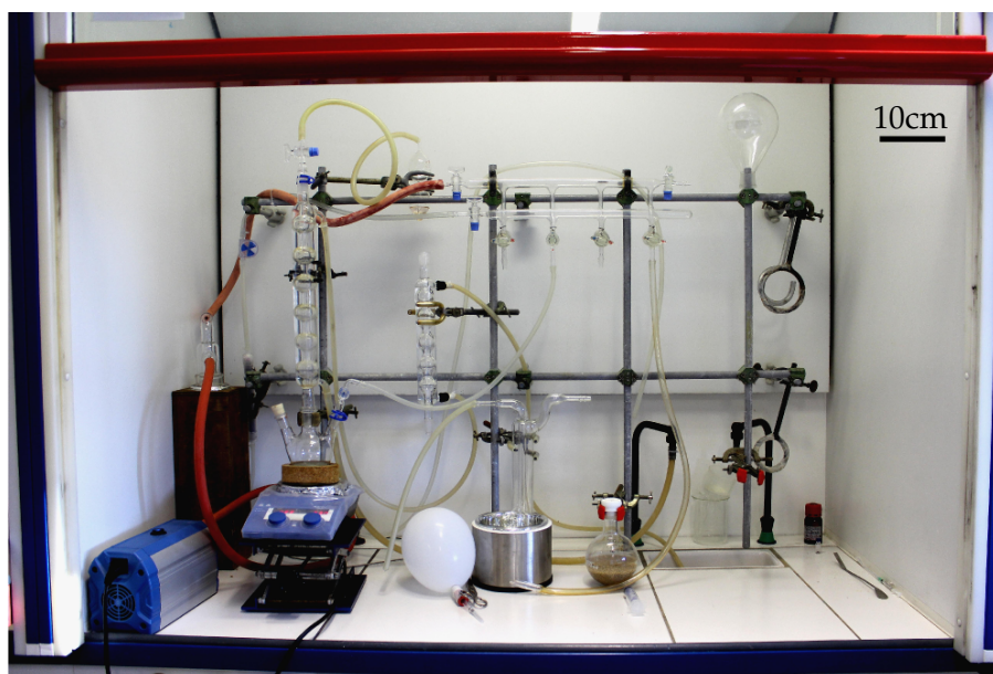
Figure 3.13: Schlenk line for the work under inert atmospheric conditions (contrast, colors enhanced, sharpened).
