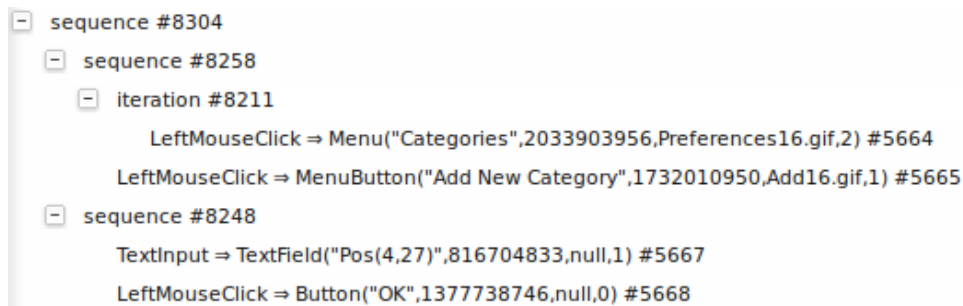
Figure 6.10.: Example for a task tree generated for the BORG calendar in the third case study.
