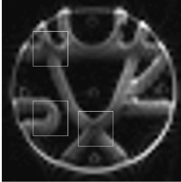
Figure 6.2: Structure of the physical phantom ( b = 0 image) with three regions of interest. ODF reconstructions of these regions are in Figures 6.3 and 6.4.
