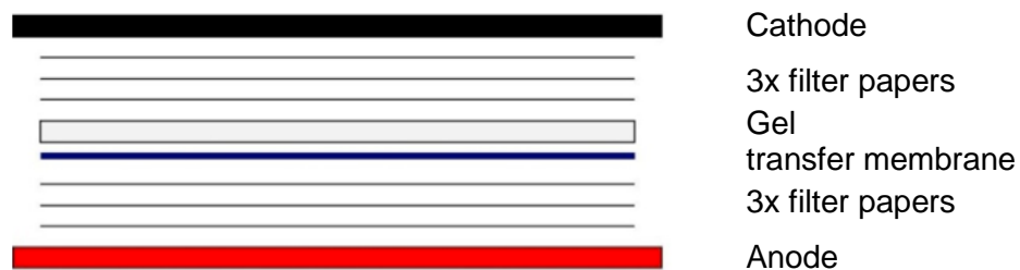
Fig. 2.1. Schematic representation of a semi-dry Western Blot “sandwich”. The Anode, positively charged, is in the lower part, the Cathode, negatively charged, in the upper part: the proteins, negatively charged, migrate downwards, from the gel to the transfer membrane
