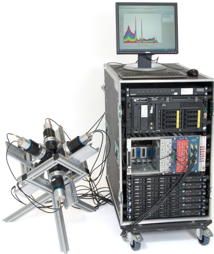
Figure 4.2: Photo of the TDPAC spectrometer with the detector holder for six detector measurements.
