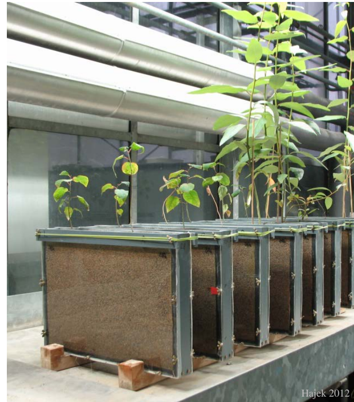
Figure A 3 Installation of the rhizobox-experiment with P. tremula and P. trichocarpa saplings, arranged in the greenhouse climate chamber of the Experimental Botanical Garden, University of Göttingen, Germany (top right). Coarse roots (a) and a young 'pioneer' root (b) of a 19-wk-old P. trichocarpa sapling growing along the observation window of a rhizobox (left). Age class (I–VI) i.e. time elapsed since first appearance (weeks) and root orders (1st and 3rd) are marked in the image.
