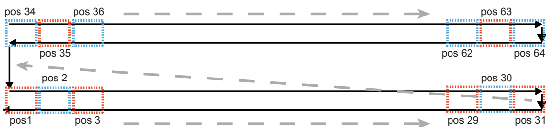
Figure 9.1: Order of the imaging process in device C. We image the drop positions in the experiments in the device C (Fig. 4.3) with a defined order. The imaging sequence positions are 1,2, ... ,64.
