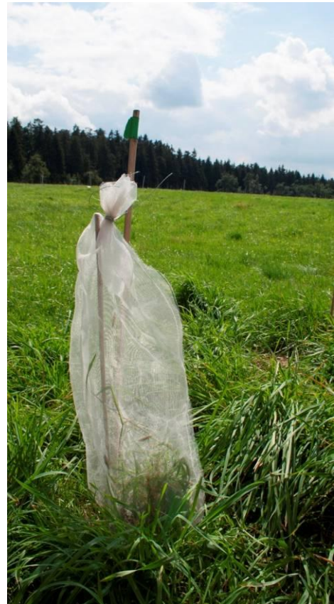
Figure 1.10: Lysimeter in the field, covered with a gauze cage.
