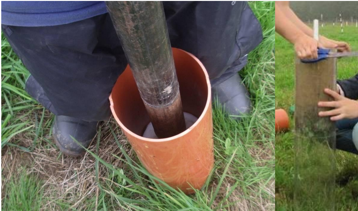
Figure 1.9: Installation of lysimeters, Right: The plexiglas cylinder of the lysimeter is stabilized using a PVC pipe whilst driving it into the ground. Left: fixing of the base plate to the lysimeter after the soil core is extracted from the ground.
