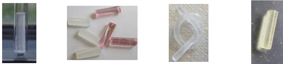
Figure 3.4: PS, PS / RAFT, PBA and PBA / RAFT sticks (from left to right).
