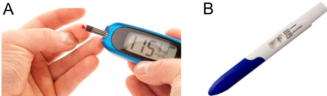
Figure 1.1.: Examples for biosensors in everyday life. A: Image of a glucometer [3]. B: Standard pregnancy test [4].
