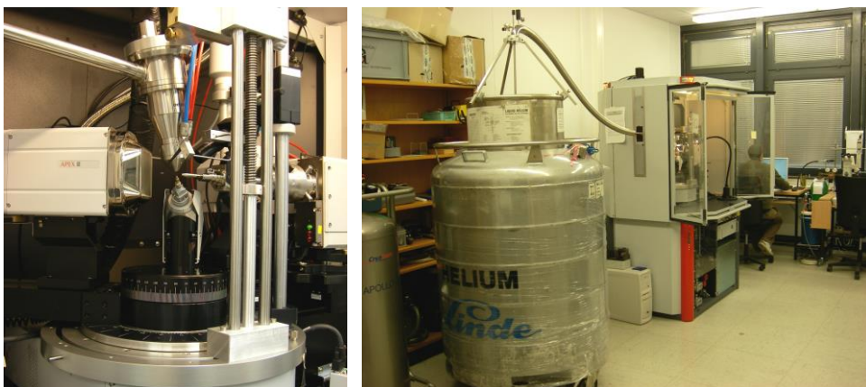
Figure 59 Measurement setup for helium-cooled single diffraction experiments on a Bruker TXS.
