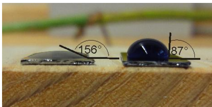
Fig. 4.12 Contact angle ( \Theta_{\text{water}} = 180^\circ - \Theta ) measurement of a water drop deposited on a hydrophilic silicon wafer (left hand side, \Theta_{\text{water}} = 93^\circ ) and a wafer that was hydrophobically functionalized with dodecyltrichlorosilane ( \Theta_{\text{water}} = 44^\circ , right hand side).
