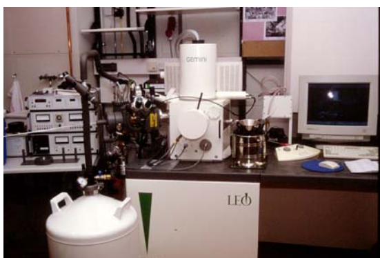
Figure 2. Picture of the cryo field-emission scanning electron microscope (LEO1530) used for the gas hydrates studies. The photo is provided by K.Techmer, GZG, Kristallographie.
