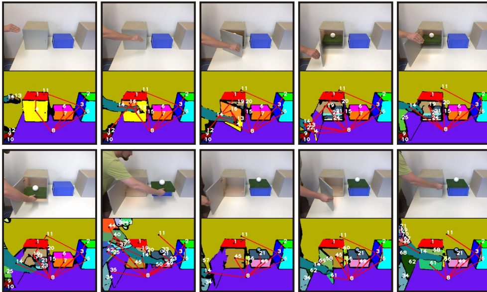
(a) First version. Cupboards are represented by at least two different graph nodes. Due to occlusion, tracking of the blue global pedestal fails while the hand is putting the tray on top.
