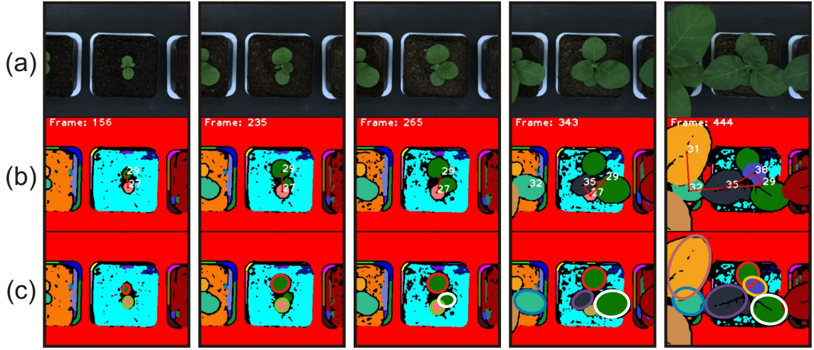
Figure 4.15: Plant sequence with merged leaf segments. (a) Original image sequence. (b) Extracted segments with corresponding graphs. Two different leaves are represented by the same segment given in green, thus, tracking of the graph node number 29 fails. (c) Fitted ellipses. In the preprocessing step edges of the new appearing leaf are detected as outliers and as the number of outliers increase from frame to frame a new ellipse shown in white is fitted to outliers.
