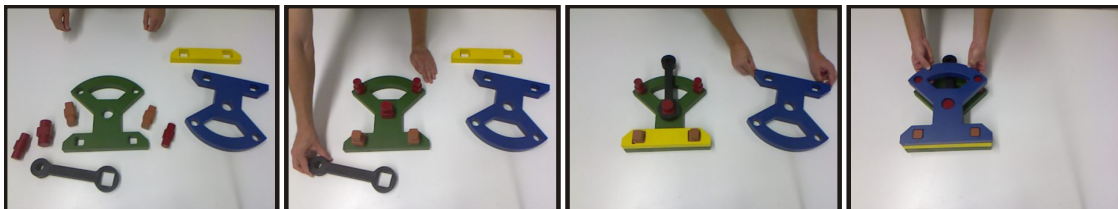
Figure 4.10: The Cranfield Benchmark (Collins et al., 1984). The complete assembly set includes two big face-plates, painted in green and blue, and a black pendulum in between. A yellow shaft is additionally needed to support the face-plates. The red and brown pegs are used to loosely connect all parts.
