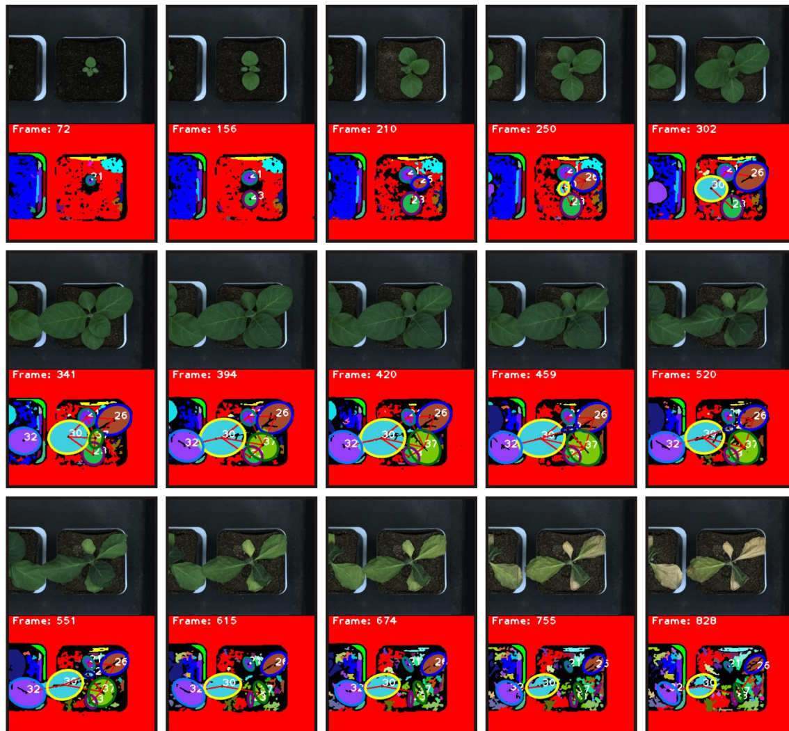
Figure 4.16: A tobacco plant sequence and corresponding segments together with extracted graphs and fitted ellipses. Graphs are continuously tracked and ellipse parameters are changing proportionally to the leaves.
