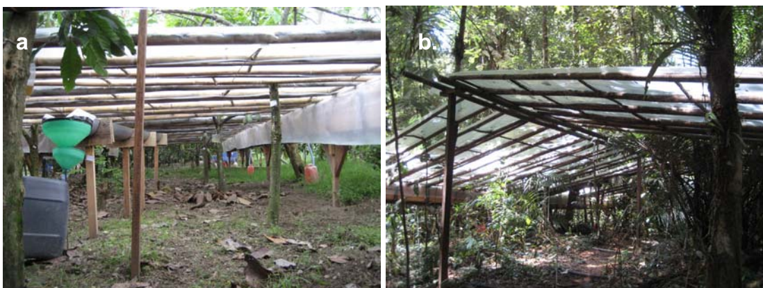
Figure 6: Pictures of the throughfall displacement roof in a) the cacao agroforestry site and b) the sub-montane tropical forest site
