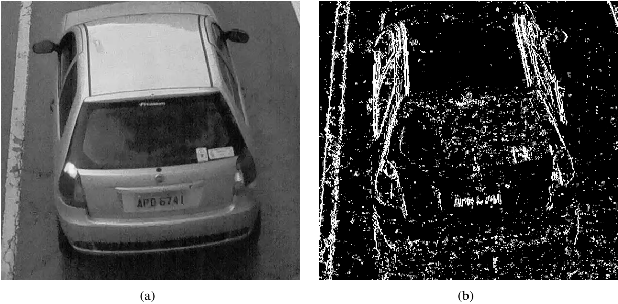
Figure 4.2: Edge extraction: (a) region of interest as given by the motion detection module; and (b) extracted edges with a threshold \gamma = 2 .
