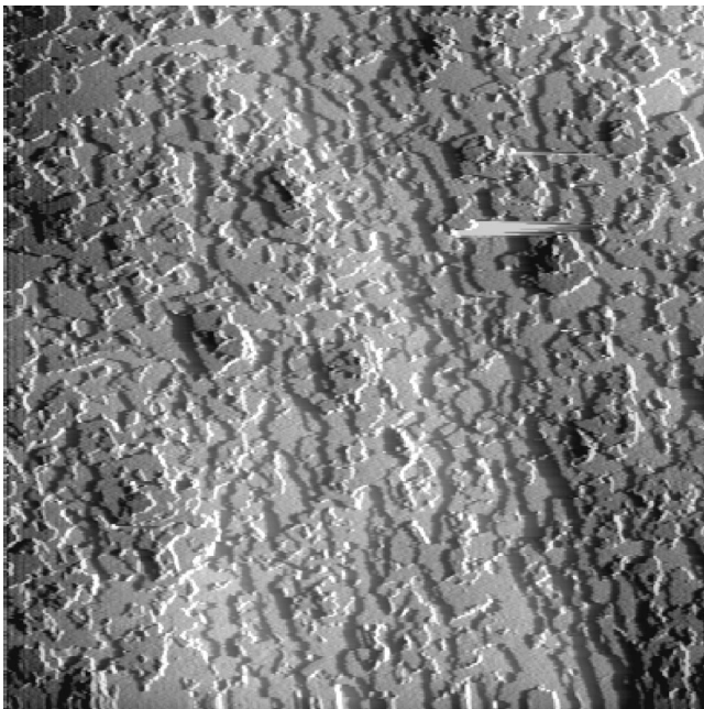
FIG. 2. STM image of a twofold surface of i-AlPdMn, size 2000 \times 2000 \text{ nm}^2 . Terraces appear, but not in a clear sequence on a large scale. At the scale of the image the picture looks rather like a landscape with mesas and flat depressions.
