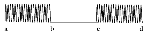
FIG. 5. Schematic of modulation applied to the pump. The pump is modulated at f_0 , the fundamental pulsation frequency, for 100 cycles between a and b, followed by a period of no modulation between b and c, followed by 100 cycles at f_0 between c and d.
