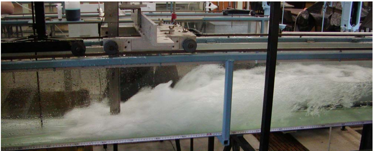
Fig. 3 – The hydraulic jump at Fr_1=14.3
