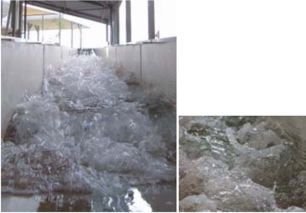
Figure 7 Advancing dam break wave down an initially dry stepped cascade ( Q(t = 0+) = 0.065 \text{ m}^3 \text{ s} , step 16, h = 0.0715 \text{ m} , l = 1.2 \text{ m} , W = 0.5 \text{ m} ), looking upstream at the advancing flood wave (left) and details of air–water flow structures (right) (Courtesy of Chye-guan Sim and Chee-chong Tan).
