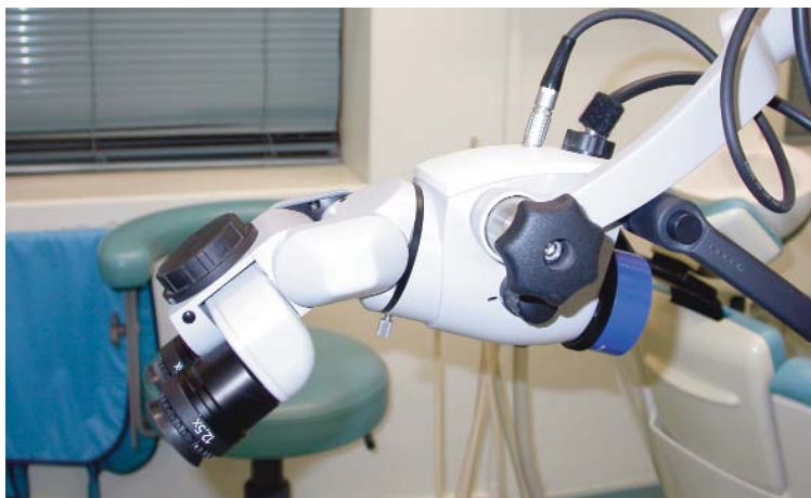
Figure 3. Typical SOM (Zeiss Pico) with video output from an internal CCD sensor and illumination supplied from a separate high intensity light source.
