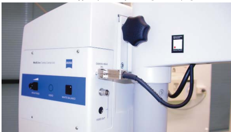
Figure 4. Composite video and S-video outputs from the SOM can be captured and/or displayed on a monitor.
