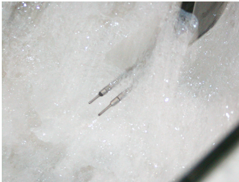
Fig. 2. Air–water flow measurements with two conductivity probes side-by-side. (A) Signal outputs in the shear layer of a hydraulic jump – transverse probe separation z = 11.5 mm, C = 0.156 , F = 136.7 Hz, y/d_1 = 0.91 , Fr_1 = 8.6 , d_1 = 0.024 m, x_1 = 1.0 m, x - x_1 = 0.2 m, W = 0.5 m. (B) Two probes separated by z = 10.5 mm, flow direction from bottom left to top right – local air–water flow properties: C = 0.79 , F = 20.6 Hz, y/d_1 = 4.15 , Fr_1 = 7.9 , d_1 = 0.024 m, x_1 = 1 m, x - x_1 = 0.2 m, W = 0.25 m.
