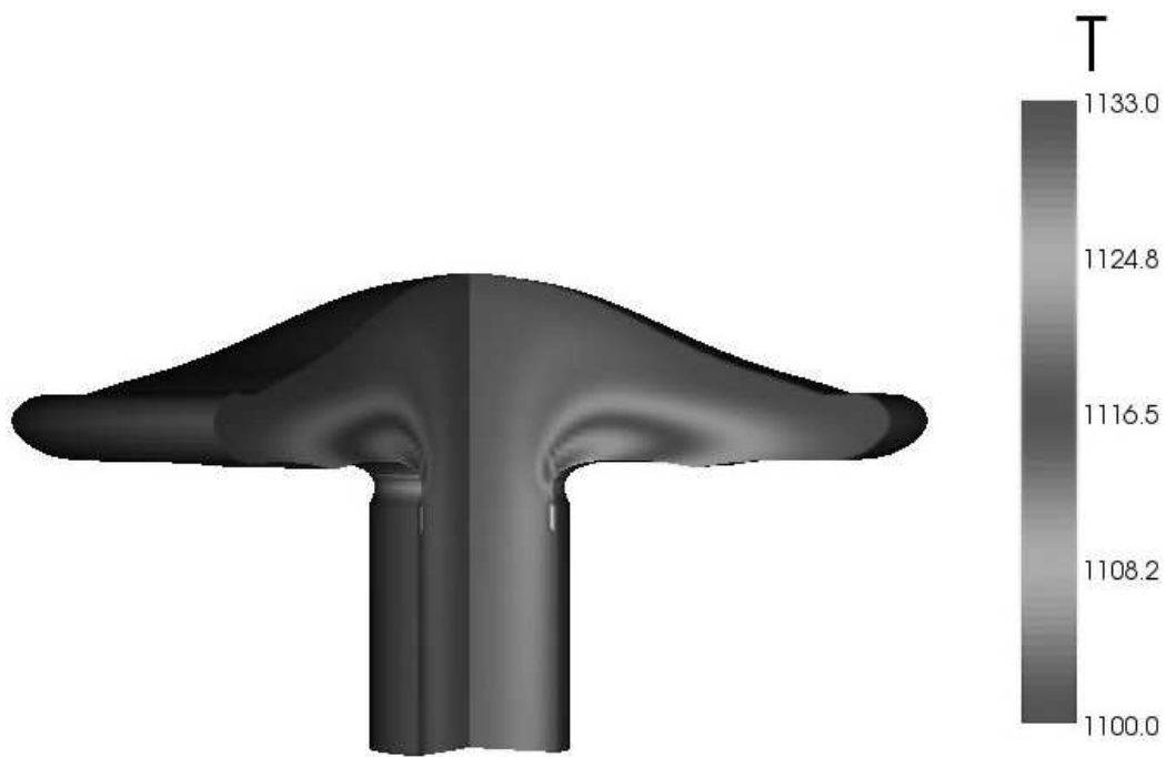
Fig. 3. Free-surface of a lava dome and upper conduit. The conduit radius is 15 m. Above the conduit the lava is free to flow on a flat horizontal plane. The cut-away region also shows the interior temperature of the lava dome as given by the scale.
