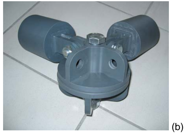
Figure 6: Prototype PVC Joint, (a) basic components, (b) assembled joint
