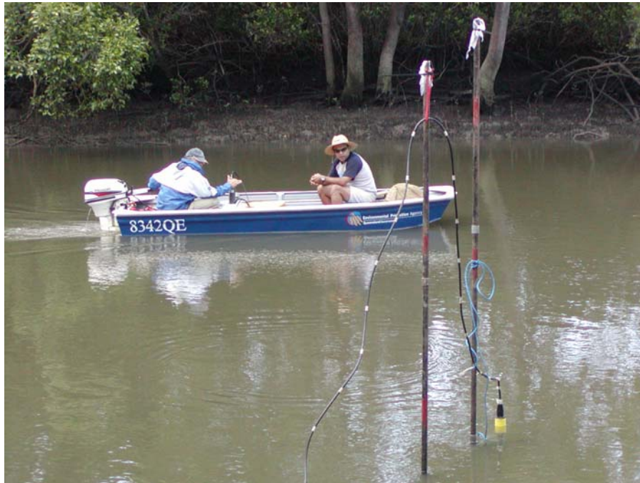
(A) ADV and YSI6600 probes at Site 2B on 24 Nov. 2003, looking from the left bank. The ADV velocimeter (yellow casing) and YSI6600 probe were held outside of the poles seen in foreground.
