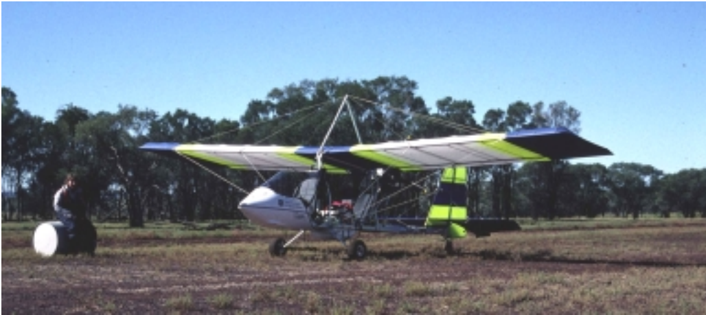
Figure 1. A Drifter ultralight aircraft set up for kangaroo survey of individual properties using line transect methodology. The observer sits behind the pilot and can count to the southern (better viewing) side in both E-W and W-E transects (Grigg, Pople & Beard, 1997).
