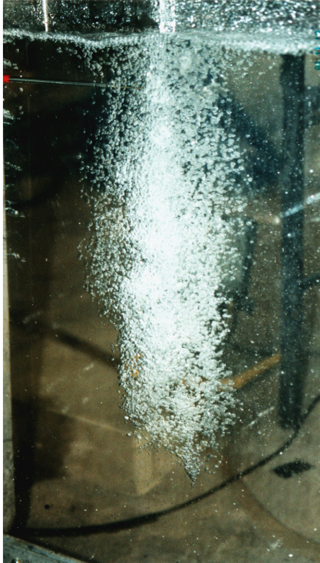
Fig. 1 - Photograph of air bubble entrainment at a vertical circular plunging jet ( V_1 = 3.3 m/s, x_1 = 0.5 m, Model 2)
