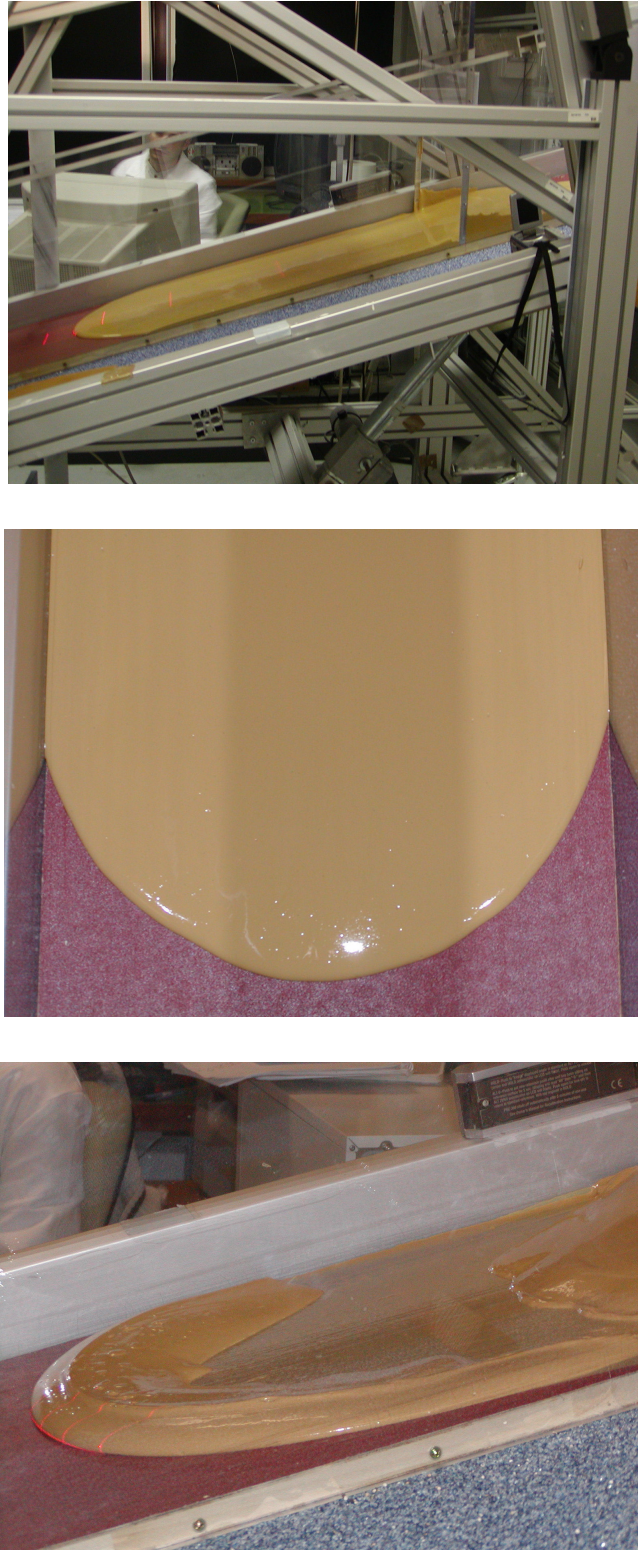
Fig. 3 Experiment with bentonite suspension (Photographs taken after fluid stoppage) - (A, Top) Flow type II, C_m = 0.15 , rest period: T_0 = 60 s (B, Middle) Flow type II, C_m = 0.15 , T_0 = 60 s, view in elevation (C, Bottom) Flow type III, C_m = 0.15 , rest period: T_0 = 2400 s, sideview of the head packet
