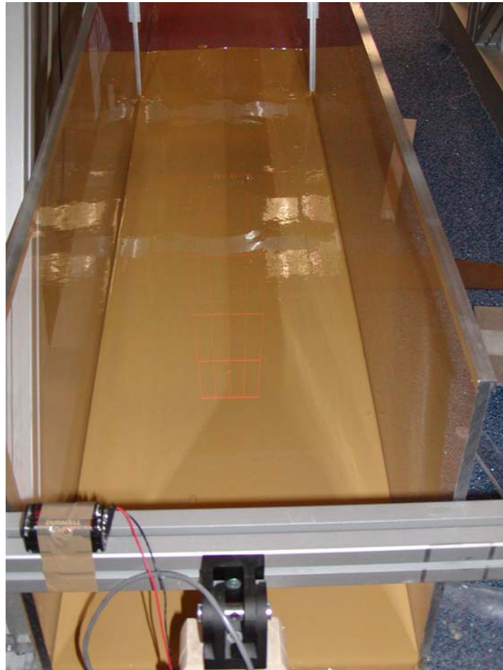
Fig. 5-1 - Photographs of Flow type I at the end of experiment - The fluid ran past the plate downstream end - Large facility (Test 23, \theta_b = 15^\circ , C_m = 0.13 , rest period: T_0 = 60 sec.)
