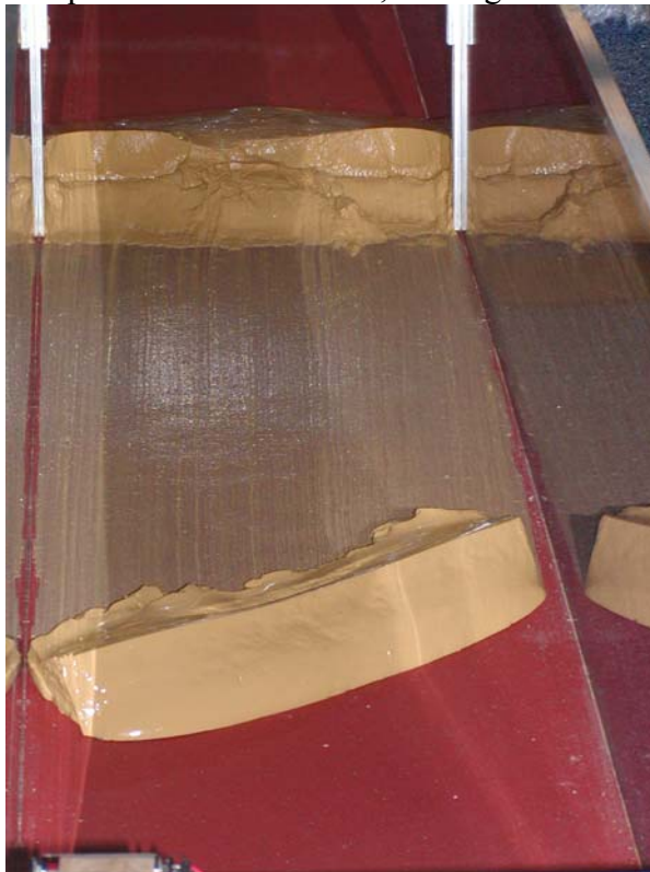
(C) Photograph of bentonite block sliding over the sandpaper after vibrating the invert (Test 26B) - Note that the block shape was quasi-two-dimensional, although it tilted around the centreline
