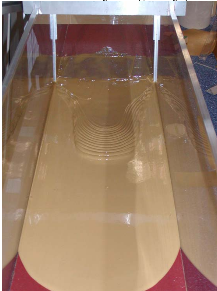
Fig. 7-2 - Man-made instabilities induced after stoppage in the large flume After fluid stoppage during some experiment, free-surface instabilities were sometimes observed during cleanup when the reservoir fluid was pushed over the stopped fluid (A) Test 05 ( \theta_b = 15^\circ , C_m = 15\% , T_o = 60 s, M = 3.7 kg, Flow Type II) (A1) Development of kind of "roll waves" during clean up, looking upstream
