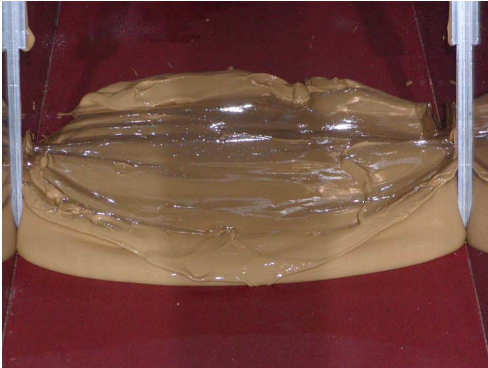
Fig. 7-4 - Instantaneous photographs of fluid motion in Flow Type IIIb Test 20 ( \theta = 15^\circ , C_m = 13\% , T_O = 17 h 16 min., M = 3.9 kg, Flow Type IIIb) (A) Second fluid packet near the downstream end of flume
