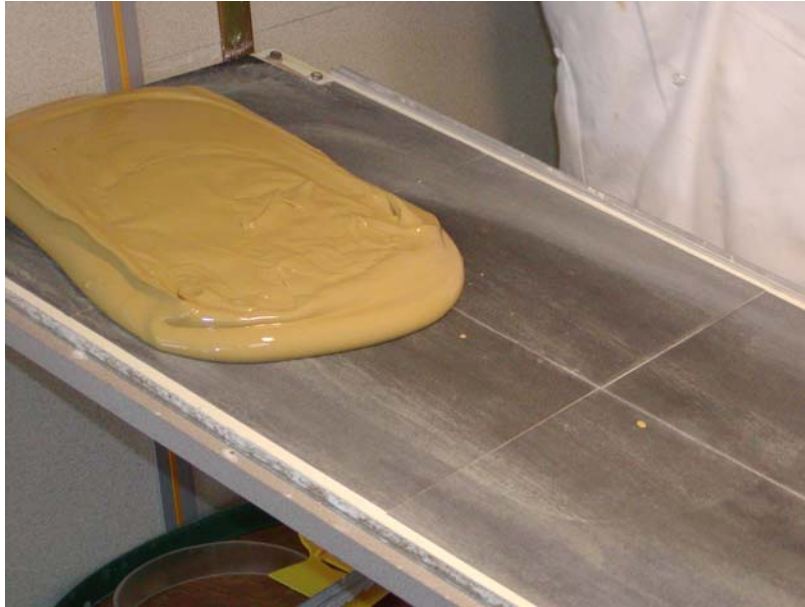
Fig. 7-2 - Man-made instabilities induced after stoppage in the large flume After fluid stoppage during some experiment, free-surface instabilities were sometimes observed during cleanup when the reservoir fluid was pushed over the stopped fluid (A) Test 05 ( \theta_b = 15^\circ , C_m = 15\% , T_o = 60 s, M = 3.7 kg, Flow Type II) (A1) Development of kind of "roll waves" during clean up, looking upstream
