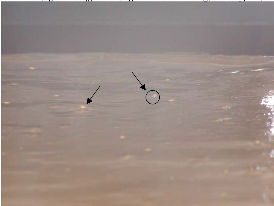
Fig. 7-3 - Free-surface details after fluid stoppage (A) Photograph showing spots of fluid restructuring at free-surface - Looking upstream at the stopped fluid - Test 06 ( \theta_b = 15^\circ , C_m = 15\% , T_O = 300 s, M = 3.7 kg, Flow Type II)
