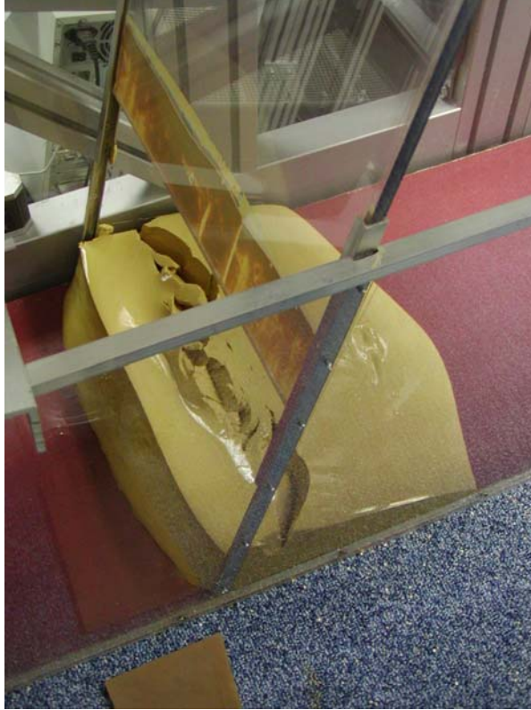
(B) Final geometry of sliding block and reservoir about 80 minutes after gate opening (Test 26)
