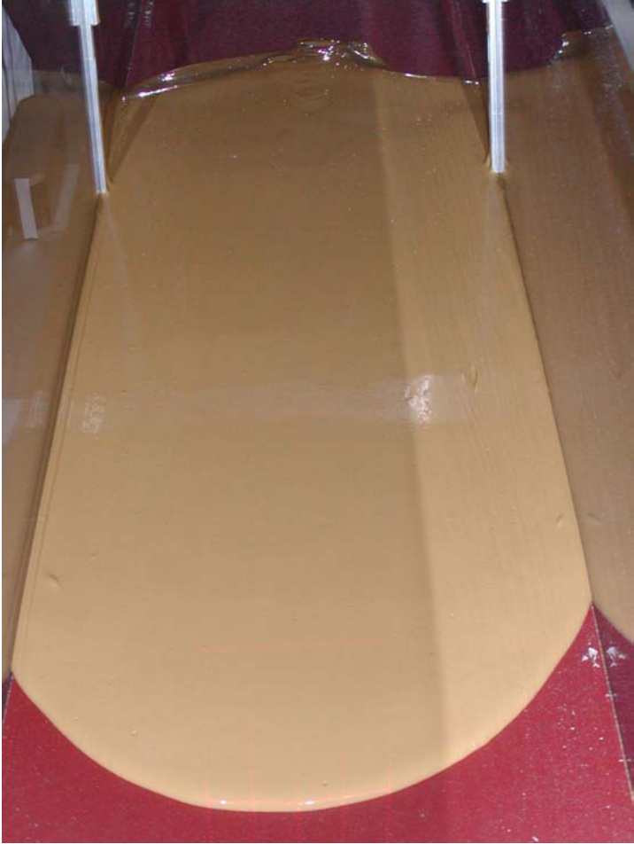
Fig. 5-2 - Photographs of Flow type II (photographs taken after stoppage) (A) Large facility (Test 04, \theta_h = 15^\circ , C_m = 0.15 , rest period: T_0 = 60 sec.)
