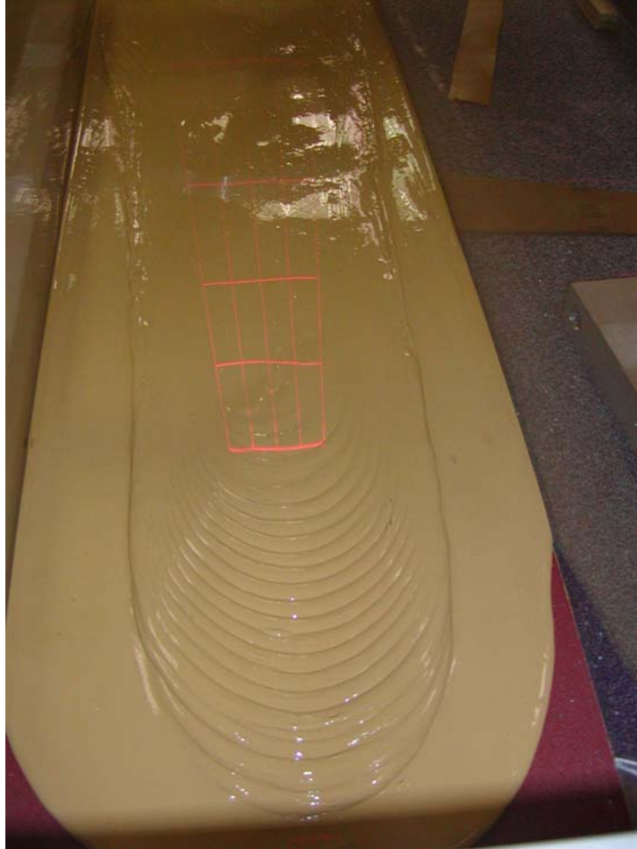
Fig. 7-3 - Free-surface details after fluid stoppage (A) Photograph showing spots of fluid restructuring at free-surface - Looking upstream at the stopped fluid - Test 06 ( \theta_b = 15^\circ , C_m = 15\% , T_O = 300 s, M = 3.7 kg, Flow Type II)
