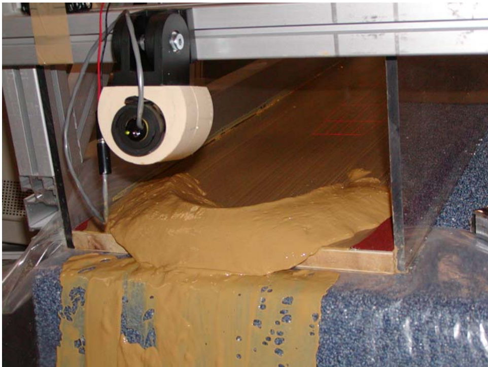
Fig. 7-4 - Instantaneous photographs of fluid motion in Flow Type IIIb Test 20 ( \theta = 15^\circ , C_m = 13\% , T_O = 17 h 16 min., M = 3.9 kg, Flow Type IIIb) (A) Second fluid packet near the downstream end of flume
