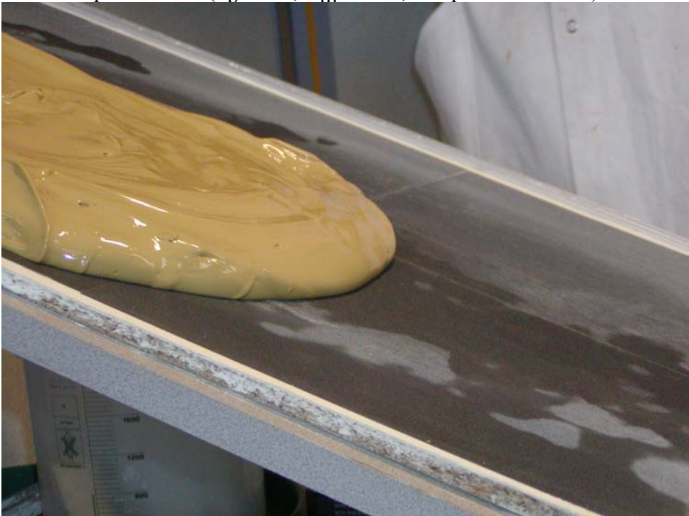
(B) Small plate with square mould ( \theta_h = 24^\circ , C_m = 0.20 , rest period: 30 min.)
