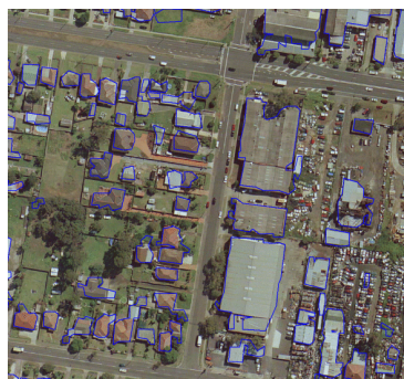
Fig. 7. Boundary polygons super-imposed to the orthophoto.
