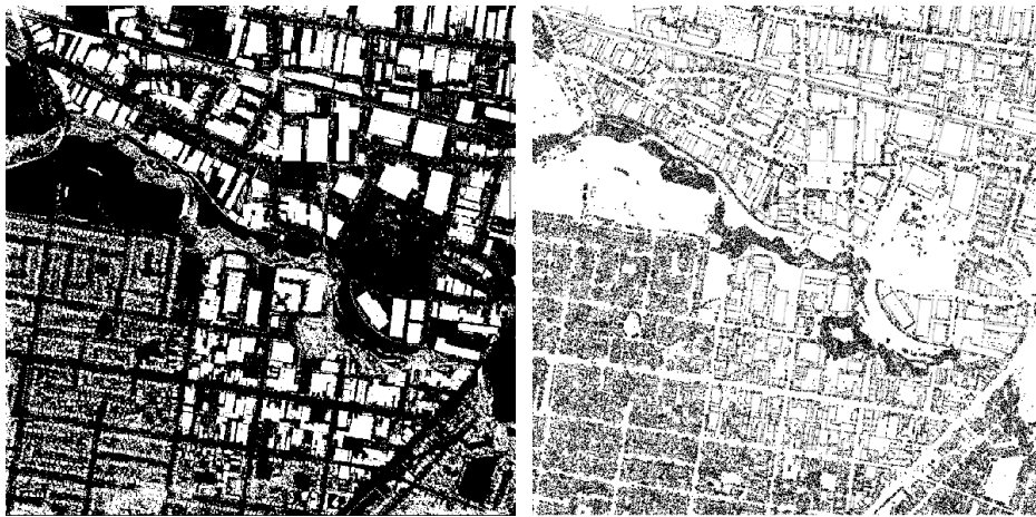
Fig. 4. The initial building mask corresponding to the left DTM in fig. 3. The residential buildings on a small hill at the southern border are merged.
