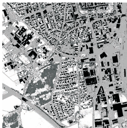
Figure 2. Initial Dempster-Shafer classification. White: grass-land, light grey: bare soil, dark grey: trees, black: buildings.
