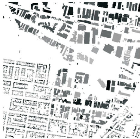
Figure 3: Buildings extracted in the third iteration.
