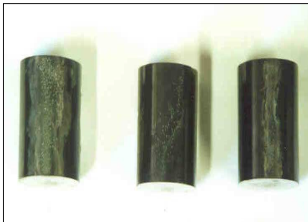
Figure 3. Surface Flash Over Tracks on Three MO Varistor Blocks
