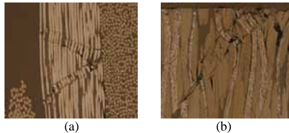
Figure 6. Micrograph of sectioned specimens; (a) Carbon fibre breakage, (b) Matrix cracking.
