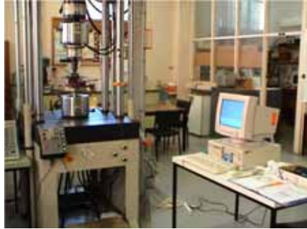
Figure 2. Pin loading setup on testing machine
