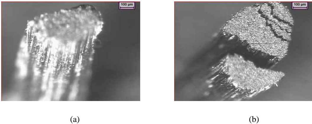
Figure 3. Optical photos of z-pin ends after DCB delamination tests in which d=0.51 mm, D=2\% ; (a) V=1 mm/min and (b) V=100 mm/min. Splitting along length of pin due to shear failure is apparent at the high loading rate. Magnification is 50x.
