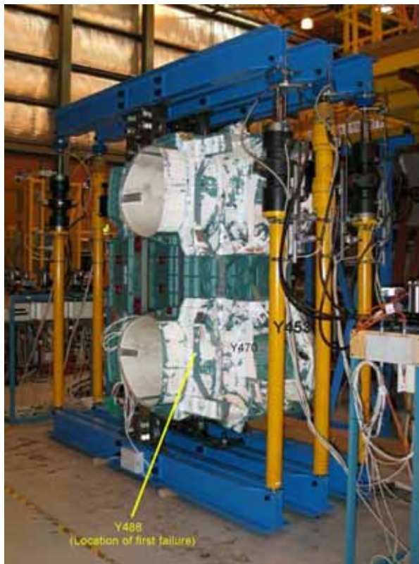
Figure 1: An F/A-18 centre barrel mounted in the FINAL rig (location of first failure highlighted)
