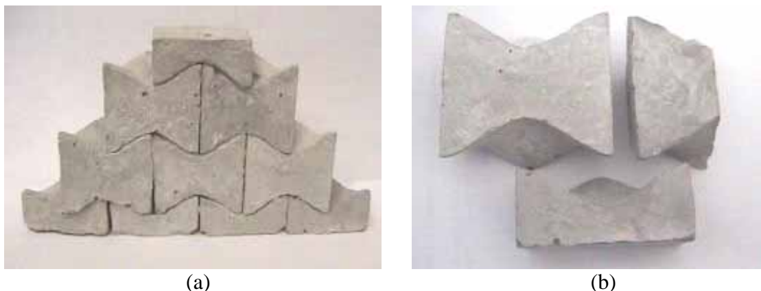
Figure 1: Osteomorphic blocks: (a) plate-like structure; (b) full osteomorphic block and two types of half-block necessary to furnish the edges.
