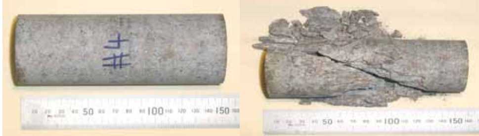
Figure 3. A UCS sample before (left) and after (right) the test
