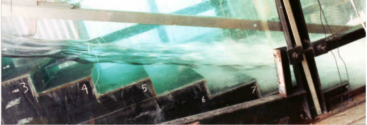
Fig. 3-1 - Views of the experimental test section (A) Skimming flow ( d_c/h = 1.5 ) - Flow from left to right
