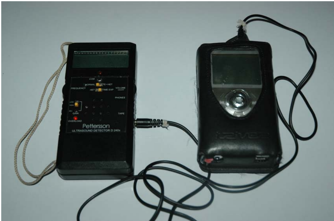
Fig. 12: Pettersson ULTRASOUND DETECTOR D 240x (left), and iHP-120 Recorder (MULTI-CODEC JUKEBOX) (right).
