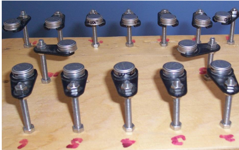
Figure 2.2 Maxim Thermochron IButton sensors used in the sensor network of 39 sites in this study.
