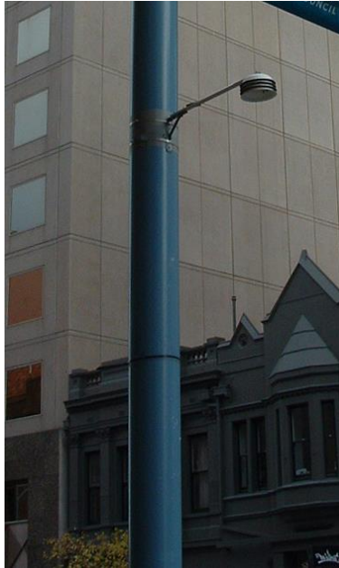
Figure 2.3 A typical CBD temperature measuring site, with the sensor inside a louvred radiation shield placed at the end of a mounting arm to distance it from its main support.
