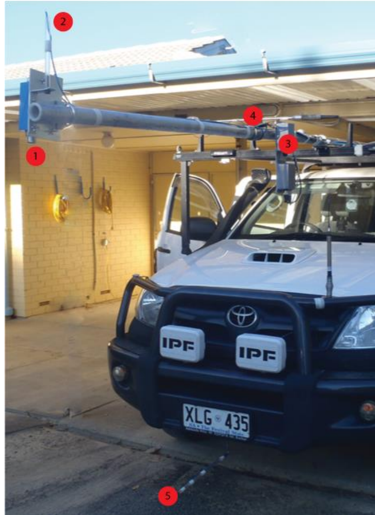
Figure 2.4. Sensors used in some night-time vehicle traverses of the CBD and suburbs. The roof-mounted boom supports (1) downwards pointing surface temperature radiometer, (2) air temperature thermocouple at 1.8 m, (3) upwards pointing sky temperature radiometer, (3) downwelling thermal radiation from whole sky, and (4) air temperature at 0.3 m, mounted on the traverse vehicle. Not shown are two relative humidity/air temperature sensors usually mounted on the boom, an air pressure sensor, and thermocouple reference sensor with its iButton comparison sensor all in a thermally isolated enclosure inside the vehicle.
